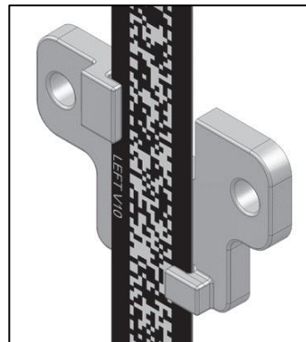
Figure 2-7: Guide Clip without Door Zone Bridge
